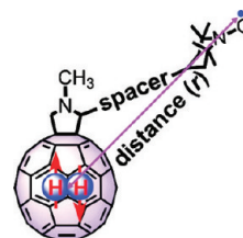
Figure 40. Schematic of the design of nitroxide spacers to determine the spin dependence of the nitroxide spin catalysis of the interconversion of the Pauli spin isomers of H_2@C_{60} .
